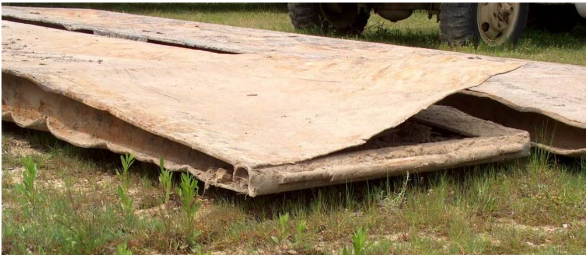
Figure 17: NCDFR Rocky Mount District Office, 2007. This bridgemat is part of the first order of steel bridgemats purchased by NCDFR in 2003. In this photo, the crimping damage on the I-beam flanges, along the end-ramp, is visible. Also, a number of bridgemats from this purchase order exhibited a breakage of the welds that bonded the top sheeting with the structural I-beams, as seen above. After welding to re-connect the top sheet, the bridgemats were placed back into service and remain in-service in 2009.
