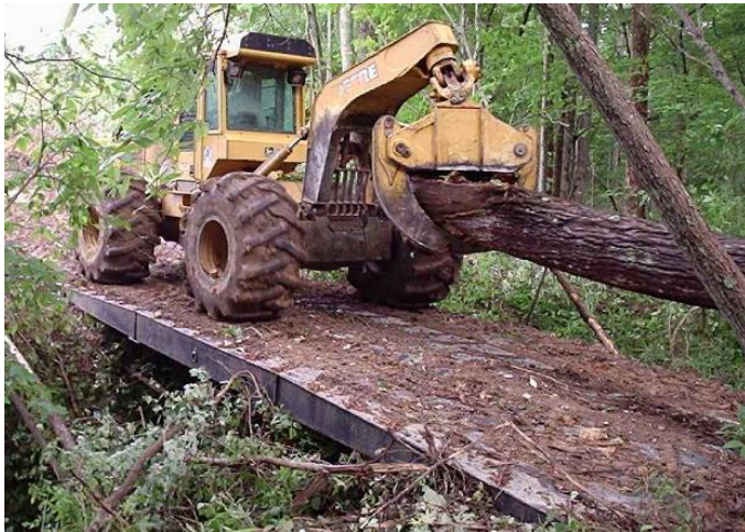
Figure 11: western North Carolina. This bridgemat appears to consist of one single panel, with tapered ends. No other information is known, but it is yet another example of the variety of ways to cross a stream by using a portable bridge.
