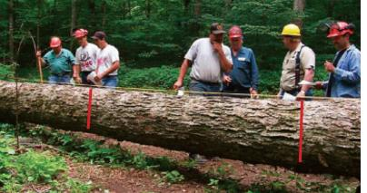
A 12' log with 20" s.e.d., 4 side clear log above an 8' 21" s.e.d., 3 sided butt log.
