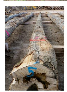
Multiple clear logs above defective butt.
