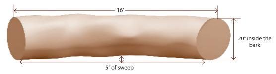
Sweep reduces the scale volume of the log. A 5" sweep can reduce log volume by 20-25%, depending on the small end diameter and log length.
