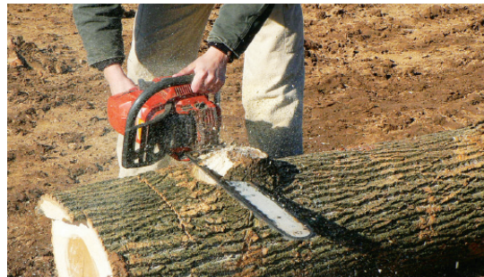
Cut knots flush with stem.
