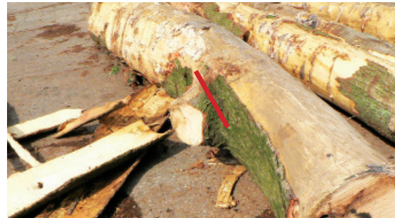
Note untrimmed knot and excessive sweep.
