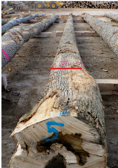
Multiple clear logs above defective butt.
