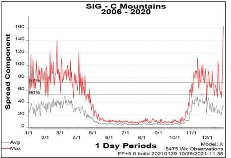
**Spread Component (SC)** - A rating of the forward rate of spread of a head fire. It integrates the effect of wind, slope, fuel bed and fuel particle properties. The daily variations are caused by the changes in the wind and moisture contents of the live fuels and the dead fuel moisture time lag classes of 1, 10, and 100 hour. *The higher the SC, the less likely that direct attack at the head of the fire will succeed.*
