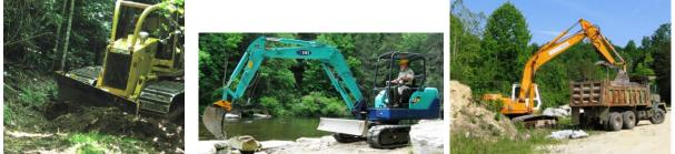
Left: A medium bulldozer with a 6-way blade. Center: A mini-trackhoe. Right: A medium, tracked-excavator with mechanical thumb, and a dump truck.
