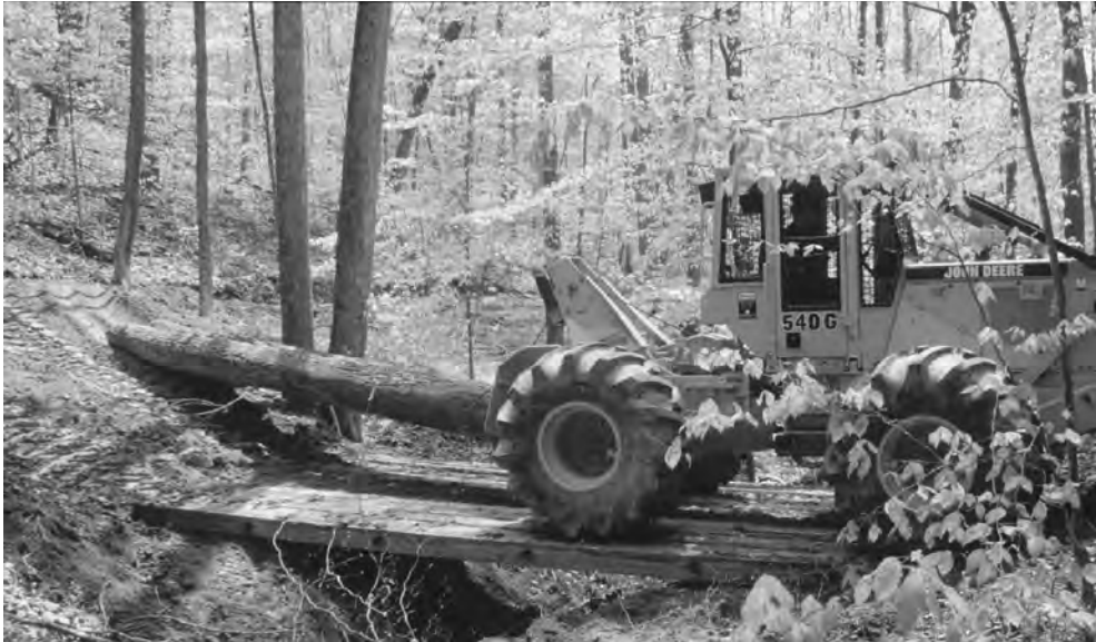
A low cost portable skidder bridge in Eastern Kentucky
