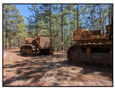
Heavy machinery located on sandy soil that is dry enough to support the equipment weight without rutting.
