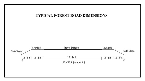
**Figure 1.** Dimensions of a typical forest road constructed in wetlands. In general a top width of 18 - 22 ft., made up of a 12 - 14 ft. wide travel surface with 3 - 4 ft. shoulders on either side, should be sufficient. Road heights of 1 - 2 ft. with 2:1 side slopes will result in total widths of 22 - 30 ft.
